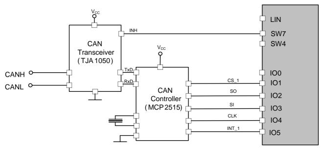
Figure 5 - Connection to external CAN controller
