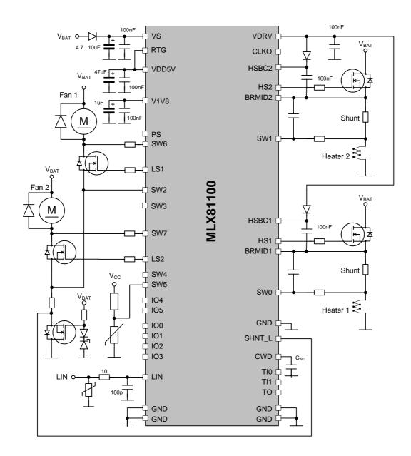
Figure 8 - Application circuitry for seat heating and seat climatisation
