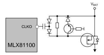
Figure 4 - High side N-FET reverse polarity protection
